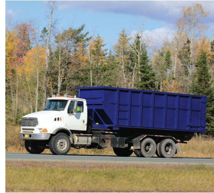
Transroulier (roll-on roll-off) Photo : iStock
